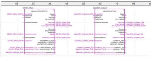
LV power device function block
